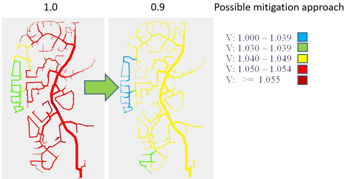
Figure 13: Example overvoltage reduction due to the reduced circuit power factor.
