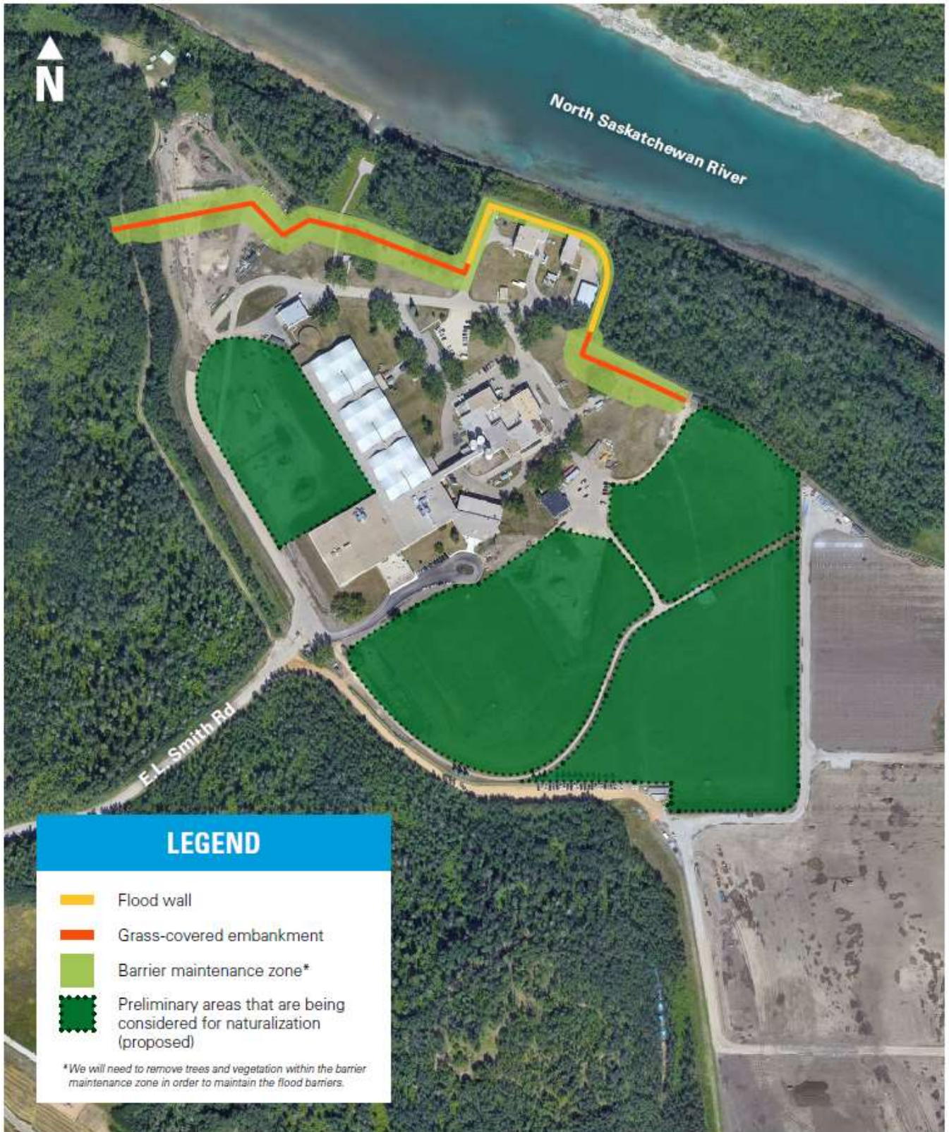
Figure 4: Infographic of EL Smith WTP plant site showing the expected impact from the flood hardening project and preliminary areas that are being considered for naturalization.
