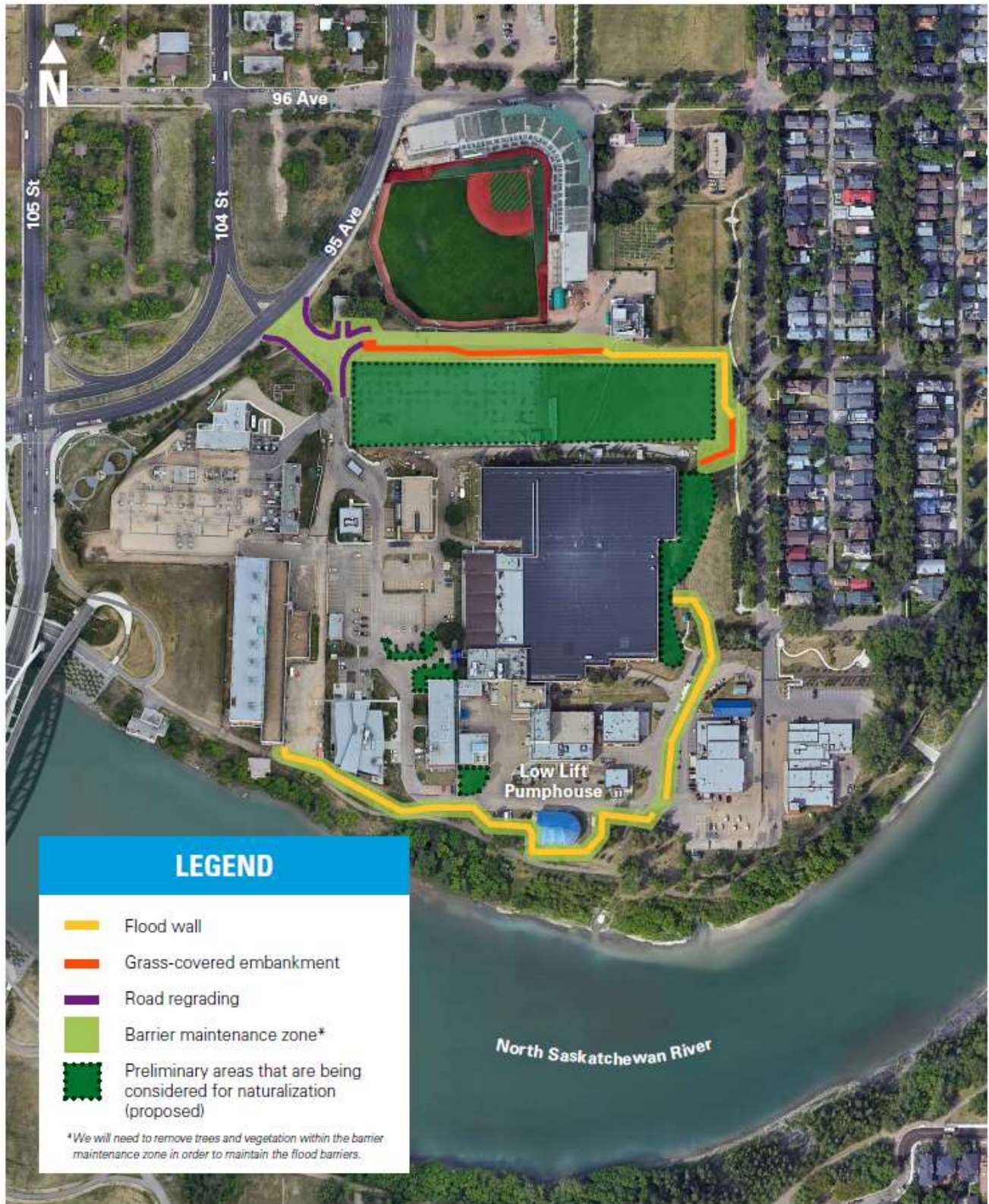
Figure 5. Infographic of Rossdale WTP plant site showing the expected impact from the flood hardening project. Pockets of naturalization are proposed to occur around the plant site over time, such as at the areas marked for naturalization on the map.
