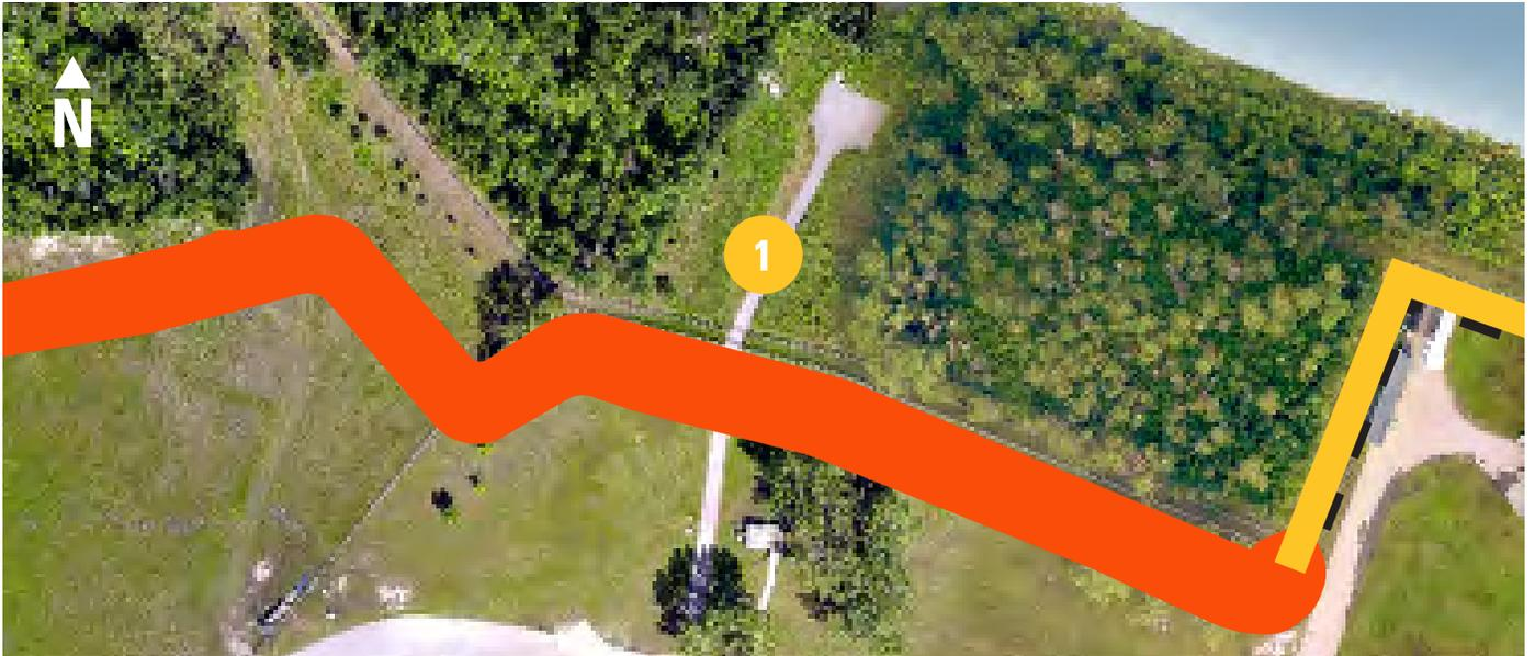
A grass-covered embankment was chosen for this location to keep the area looking more natural, and because there is space to accommodate it within the existing fenceline. There will be some trees and vegetation removed on the water treatment plant side of the fence in order to construct the embankments and allow for a buffer zone. The trees could be replanted within the water treatment plant site.
