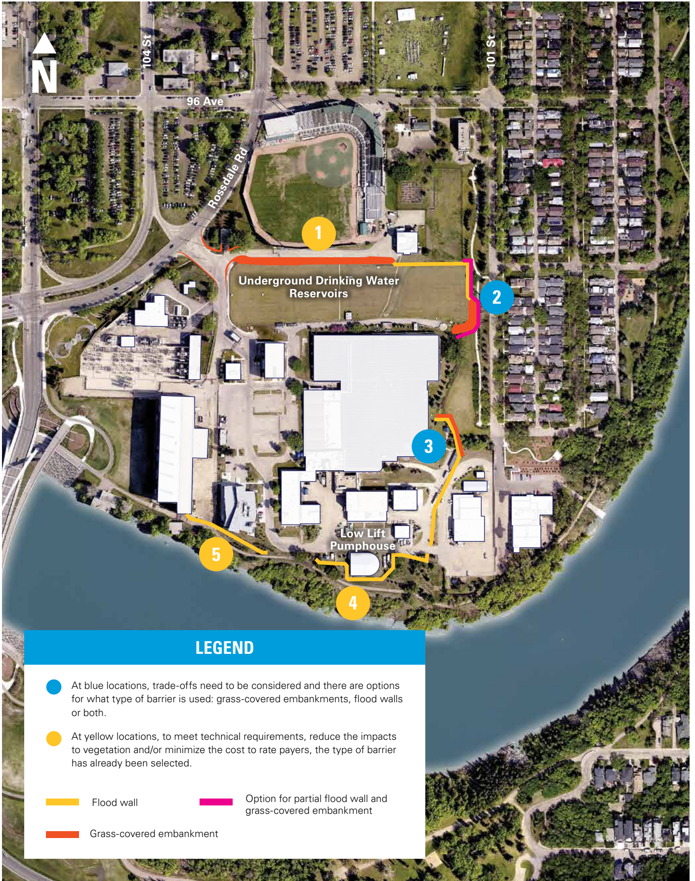
Map updated April 2022 to show revised design at location 4. A wall has been selected for this location due to engineering requirements.
