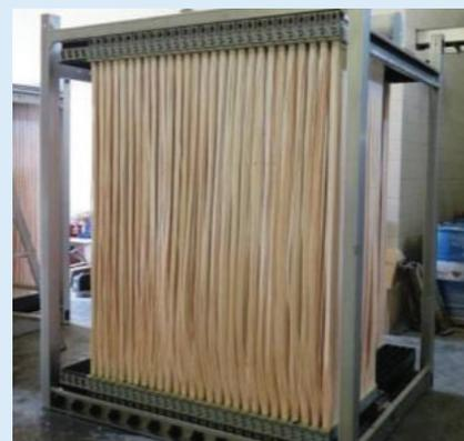
Membrane technology that would be inserted into existing tanks.
