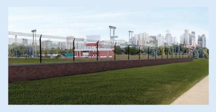
With either type of flood barrier (wall or grass-covered embankment) buffer zones are in place that restrict the type of vegetation that can be replanted. The buffer zone is about 5m from the wall or end of the embankment slope. This is to maintain the structural integrity of the barrier.
