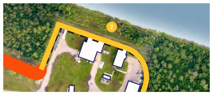
A flood wall was chosen for this location. The wall will range from 2.5 to 4.5 metres tall depending on the contour of the ground. A wall here would protect the critical river water intake infrastructure, while minimizing the impact to the wildlife corridor between the river and the water treatment plant. The space between the flood wall and the trees could be planted with local grasses.
