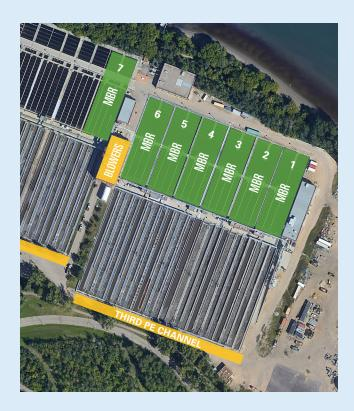
Starting in 2027, EPCOR will start retrofitting existing secondary clarifier tanks with membrane technology.
