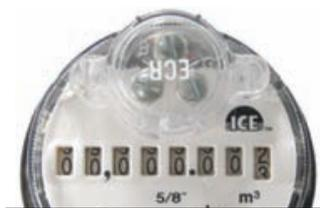
An eight-dial meter records water usage in cubic metres to the nearest 1/1000.
